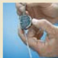
Thread locking device onto cable
