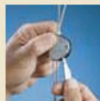
Release cable with unlocking tool or small screwdriver
