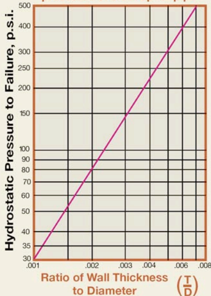
Chart to predict bursting pressures of steel Spiral pipe
